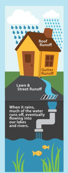
When it rains, water collects on our driveways, sidewalks and yards. Some of it is absorbed into the ground, but most of it flows into storm drains, then to pipes under the street and finally into a river or lake. (We call this water 'runoff' or 'stormwater'.) As it runs off, the water mixes with pollution that's on the ground - litter, chemicals, and animal poo, to name a few! *Ewww, right?*
